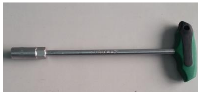
Fig. 4: Socket-wrench with T-handle (wrench size 4mm)
